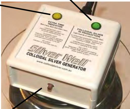
This switch adds EXTRA TIME that will commence once the Auto mode has completed its cycle. Each click adds 1 hour. You can add extra time any time the generator is operating with the right hand light illuminated. (To use the generator in IMPURE WATER you MUST add EXTRA TIME before the electrodes are lowered into the water. See page 9 for more in this).
